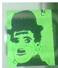
Fig.2: OLED performed by localized ITO etching (black area) with SECM
